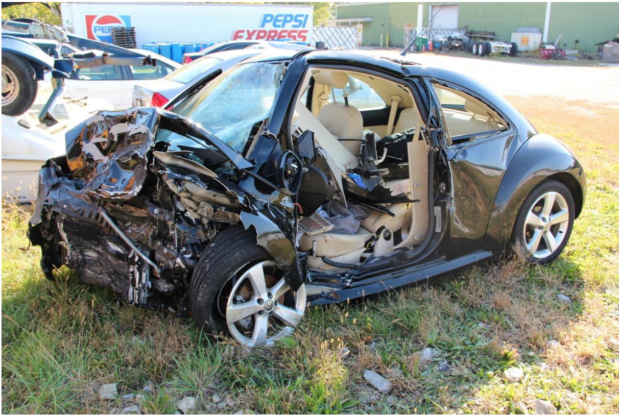
Figure 9. Damage to the wrong-way vehicle from the Beloit, Wisconsin, collision.
